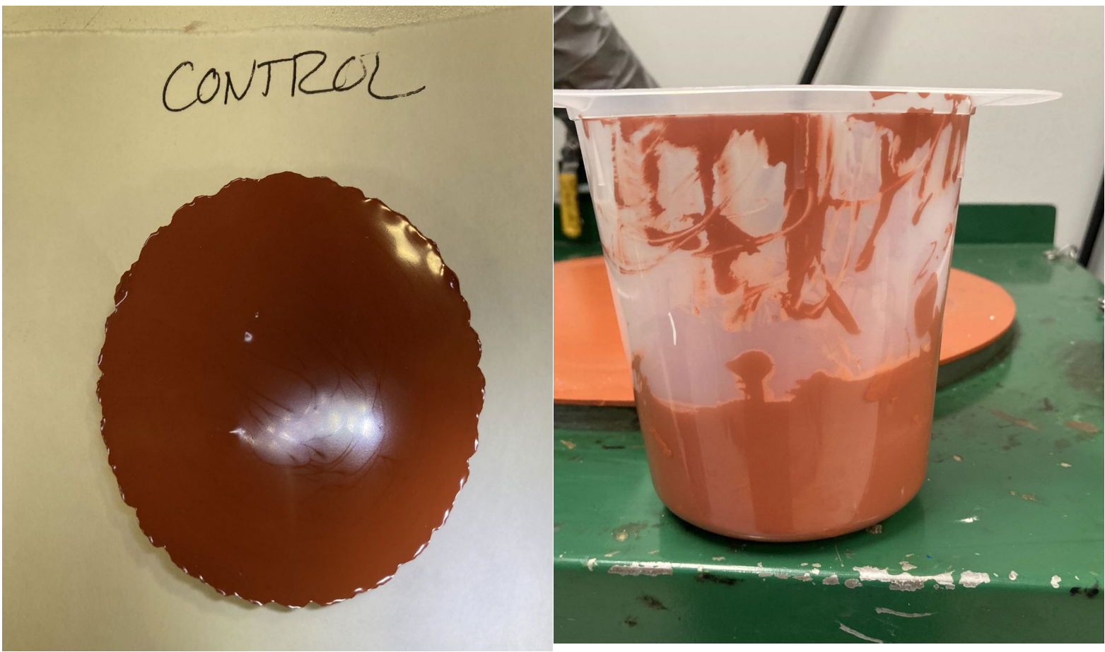
Figure 3. Silicone Puck that was put through testing (left) and the silicone before being mixed (right)
